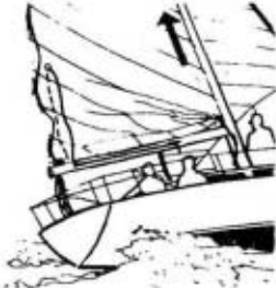
2. The main halyard is tightened up. Note: The mainsheet should be stacked only if necessary. (Usually when releasing).
