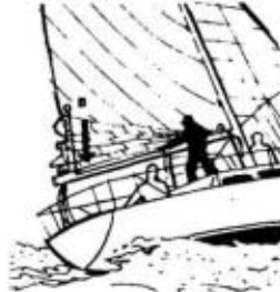
3. The reef clew outhaul (B) is tightened up to the reef cringle and cleated. With practice, a Quick Reef can be executed in between 15 and 30 seconds on a boat of 40' (12.2 m) in length!
